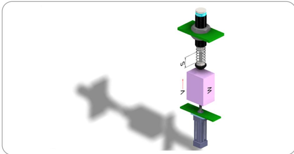
ex. 6 Horizontal Impact with Motor Driving
