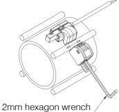
Step 2 Use 2mm hexagon wrench to lift up the screw cap to remove the retaining bracket.
