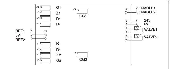
If ENABLE1 is connected 0V, VALVE1 can give output signal. If ENABLE2 is connected 0V, VALVE2 can give output signal. CG1,CG2 current trimpots G1,G2 gain trimpots Z1,Z2 zero trimpots
