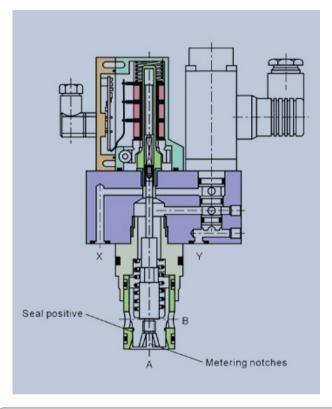
Series QPG-16/50 Cartridge Proportional Valves with external valve amplifier DIN 24 342, ISO/DIS 7368 Pilot operated 2/2 directional control cartridge valve.
