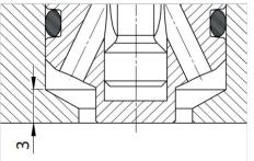
The nose of the valve protrudes by 3mm into ID 10mm of the cavity.
