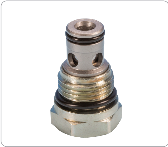
SAE08 Cartridge-420 bar Direct acting-Poppet Type
