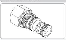
When pressure at ① rises above the selected spring bias pressure against the spool, the valve shift to allow flow from ① to②. Pilot pressure at ③ is additive to the spring bias pressure. The valve may be used in switching or conpensation type applications.
