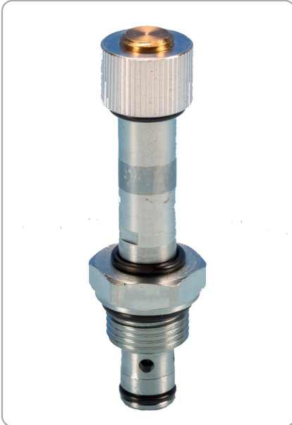
Hybrid SAE Cartridge - 250 bar NC Double Lock Direct Acting - Poppet Type
