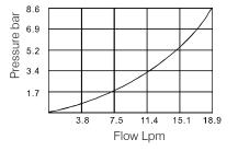
Shuttle Valves, cartridge-style hydraulic check valve, for use in blocking circuits where a priority of flow / direction is given to a higher pressure circuit over a lower one. A load - shlutting.
