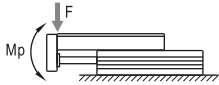
6.1) Table deflection due to pitch moment: Table deflection (arrow) when a load acts upon the section marked with the arrow at the full stroke of the compact slide.
