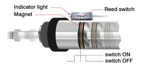
When the piston's magnet approaches the magnetic sensor, the internal reed switch will detect the change of magnetic field and close the contacts.
