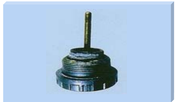
■ Rust of valve parts
