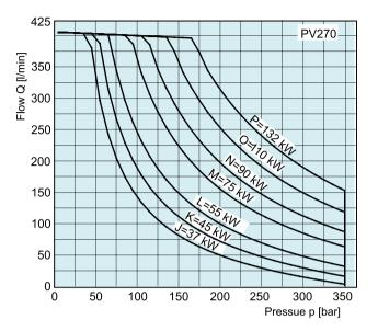
he diagrams are only valid for the following working conditions: speed: n=1500 ( - - -) and 1800 ( - - -) rev/min temperature: t=50°C fluid: mineral oil HLP, ISO VG46 viscosity: v=46 mm2/s at 40°C
