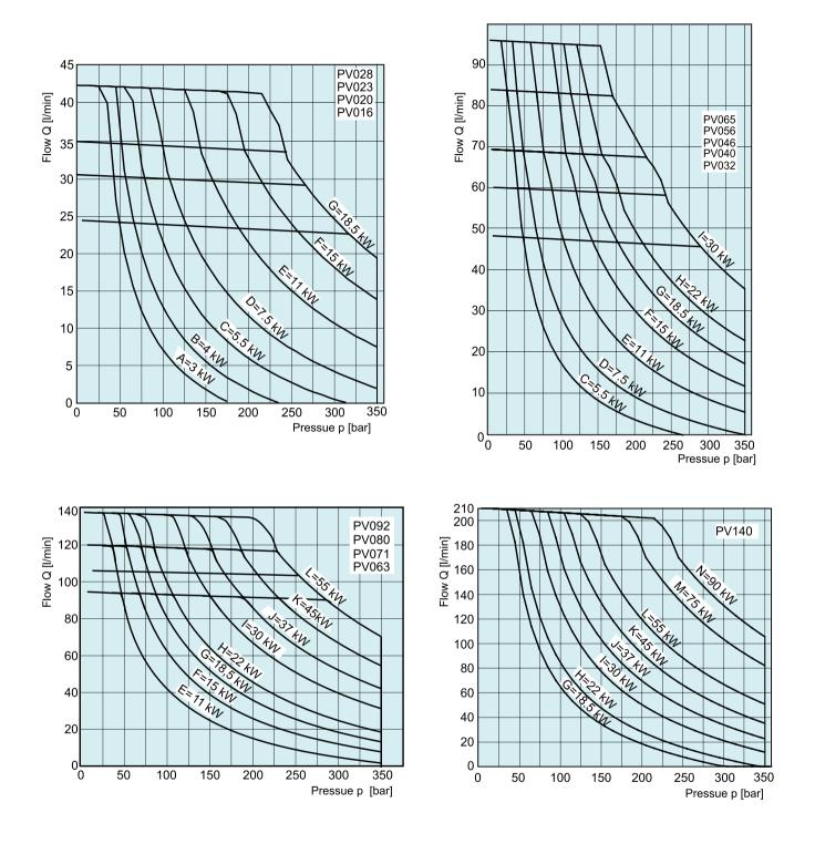
The diagrams are only valid for the following working conditions: speed: n=1500 ( - - -) and 1800 ( - - -) rev/min temperature: t=50°C fluid: mineral oil HLP, ISO VG46 viscosity: v=46 mm2/s at 40°C
