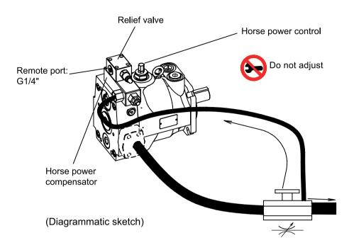
PH Horse power load-sensing compensator + Relief valve
