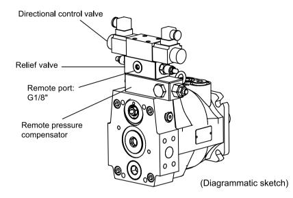
GC Remote pressure compensator + Electrical unloading + 2-stage pressure control
