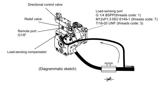
HR Load-sensing compensator + Electrical unloading
