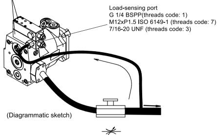
VM 2-valve load-sensing compensator with NG6 interface
