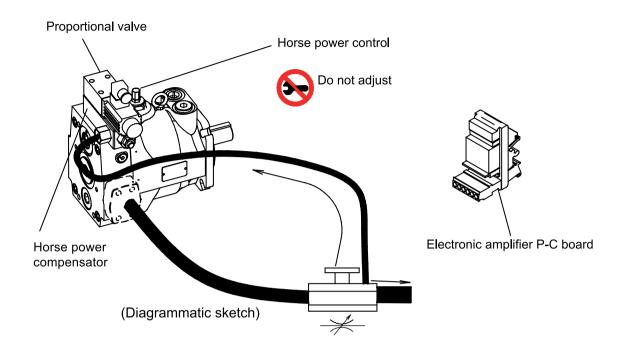
PS Horse power load-sensing compensator + Proportional pressure valve
