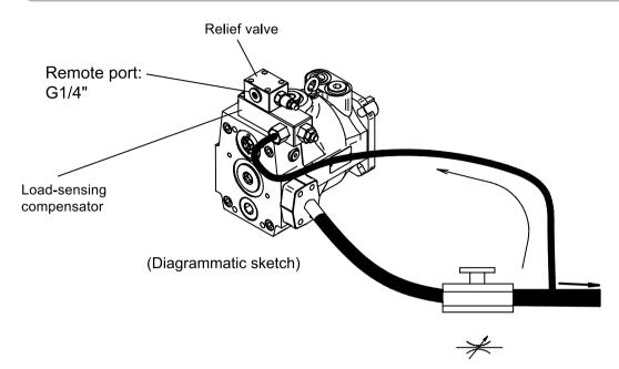
HA Load-sensing compensator + Relief valve
