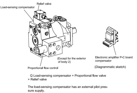
Factory setting for the differential pressure is 10bar. The input signal to the compensator is the differential pressure at the main stream resistor.
