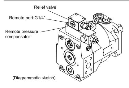
GA Remote pressure compensator + Relief valve
