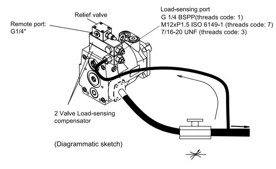
VA 2-valve load-sensing compensator + Relief valve
