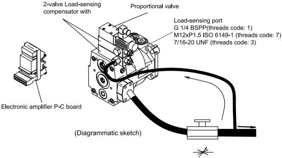
VJ 2-valve load-sensing compensator + Proportional pressure valve
