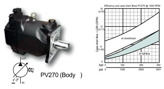
The efficiency and power graphs are measured at an input speed of n = 1500 RPM, a temperature of 40°C and a fluid viscosity of 46 mm2/s.
