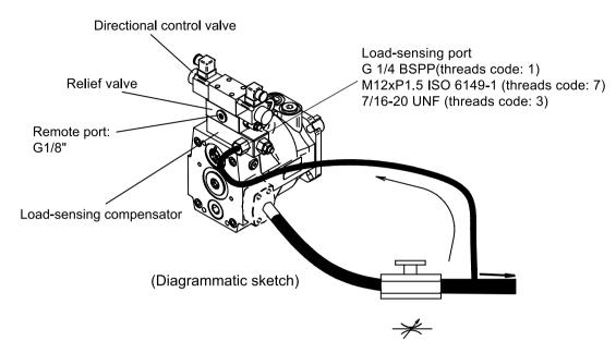
HC Load-sensing compensator + Electrical unloading + 2-stage pressure control
