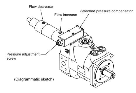
one-stage flow compensator (Cylinder)
