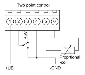
. Clamp connections plug in connector Pin 1 =+ UB; supply voltage (10-35 VDC)
