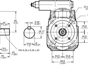
30.2 (1.19) Inlet: -flange according to ISO 6162 DN 32 ; PN 250 bar 58.7 (2.31)
