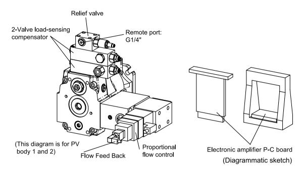
FV 2-valve load-sensing compensator + High reacted proportional flow valve + Flow feed back + Relief valve
