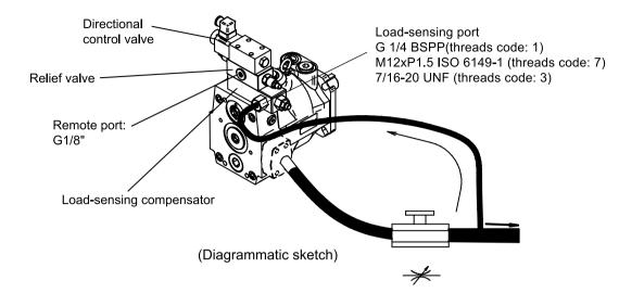
HB Load-sensing compensator + 2-stage pressure control
