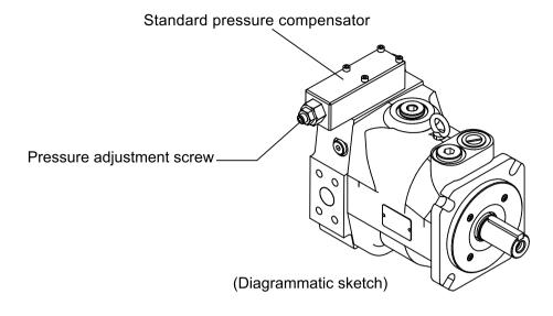
A0 Standard pressure compensator
